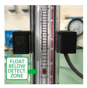
If a "high level alarm" is required, the float must be positioned below Detection Zone before powering up.
