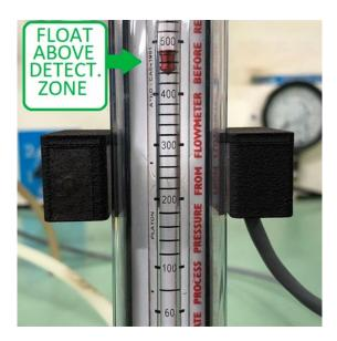
If a "low level alarm" is required, the float must be positioned above Detection Zone before powering up.
