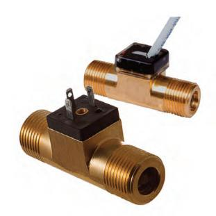
The turbine meters of the VISION® series are for the exact metering of small quantities of liquids. The actual flow as well as the flow already flowed through can be measured. The VISION® 2000 series is used for flow rates up to 35 l/min.
