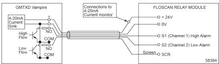
The Platon Vampire d.c. powered flow transmitter (see OMM1033) can be powered from the Floscan relay module, and the alarm outputs used to drive the relays. Note that current sensing for the flow analogue output must be in the 24V line.
