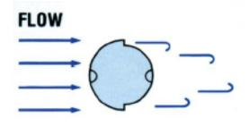
single pressure sensing port; the precision engineered profile of the Flo-Bar at this reference pressure position ensures a stable separation for flow vortices, giving a stable flow calibration factor over a wide flow turndown.
